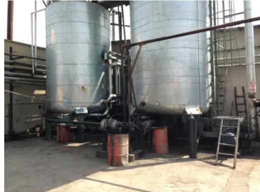
Blowing end point is usually signified by sampling from tower and bitumen properties testing. The blowing operation stops when oxidized bitumen reaches to specified properties. After this in order to fix the final point and depolymerization bitumen got in high temperature. It is necessary to be transferred to store after packing and presented to sale.
